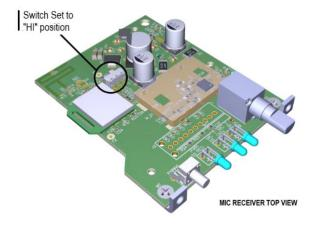
4. Attach Mic Receiver to rear panel, carefully aligning the L-brackets and LEDS with rear panel holes. Fasten Receiver with the two black long screws using a Phillips # 1 screw driver. Attach volume knob.
