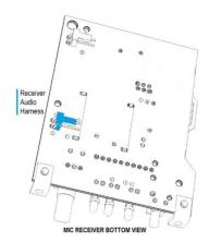
6. Connect Power Harness (Red/White or Blue/Green) to any of the three available small 2-pin header labeled "- +" located right, near the 20-pin header "CN1" on AMP PCB.
